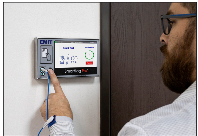
Figure 24. Performing a single-wire wrist strap test
