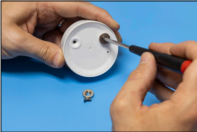
Figure 7. Installing the Desco 19344 Ring Magnets
